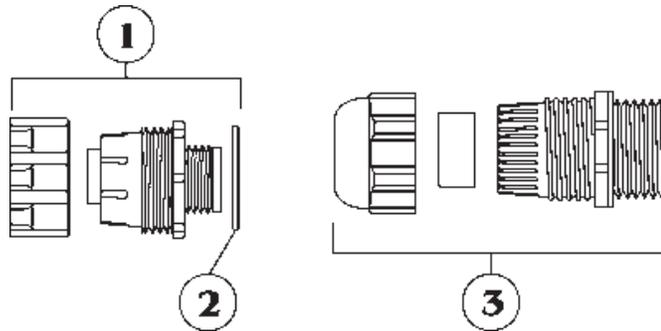
1. Armoured cable strain relief gland GR 0018
